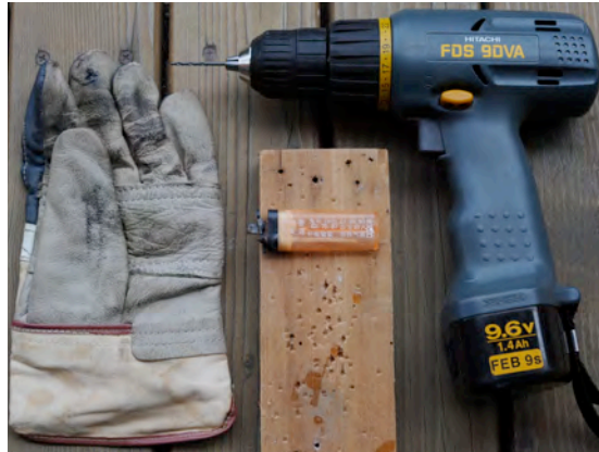
Fig.3 Tools for removing the gas from lighters
